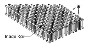
Attach the middle (if any) and top spacer bars to this side of the rack.
