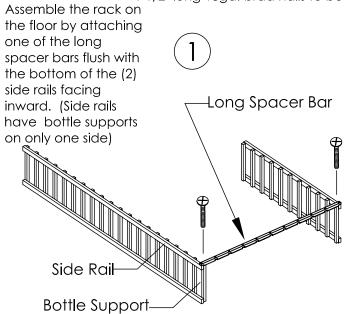
Attach the remaining rails in order to this spacer bar. Be sure to attach the spacer bar flush with the bottom row of bottle supports.
