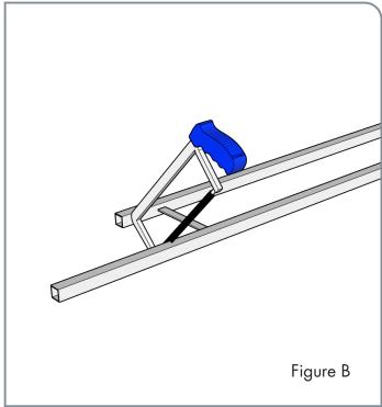
Note: An abrasive cut-off saw should not be used, as the heat generated is likely to damage the finish of a Wall Series Frame.
