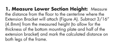
**Note:** If the calculated measurement aligns with one of the cross members, cut 2" (52mm) off the end of the frame and then mark the cut lines, measuring away from the fresh cut.
