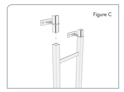
**4: Install Lower Frame:** Following the directions the W Series Frame and/or any other mounting plate instructions, install the lower end of the W Series Frame into the wall or ceiling.
