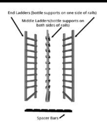
Instructions show a sample 6 column rack. All 42" Upper Racks are assembled in the same manner. Your order will contain the specific number of ladders and spacer bars appropriate for your chosen rack. Racks wider than 10 columns will have segmented spacer bars with clips to attach them together.
