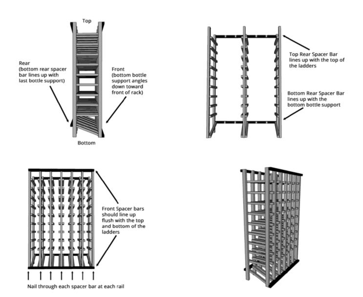
If using rack on top of a base you can nail through the bottom spacer bar of the upper rack into the top spacer bar of an assembled base rack. It is recommended you secure both racks to a wall for optimal stability. Hardware for attaching to a wall is not supplied. Simple "L" brackets from your local hardware store are a popular option for securing to a wall.
