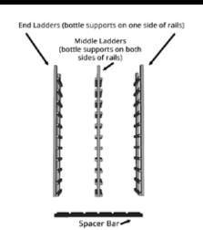
Instructions show a sample 6 column rack. All 42" Upper Racks are assembled in the same manner. Your order will contain the specific number of ladders and spacer bars appropriate for your chosen rack. Racks wider than 10 columns will have segmented spacer bars with clips to attach them together.
