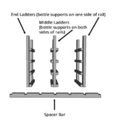
Instructions show a sample 6 column rack. All 15 3/4" Upper Racks are assembled in the same manner. Your order will contain the specific number of ladders and spacer bars appropriate for your chosen rack. Racks wider than 10 columns will have segmented spacer bars with clips to attach them together.
