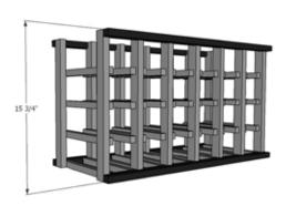
If using rack on top of a base you can nail through the bottom spacer bar of the upper rack into the top spacer bar of an assembled base rack. It is recommended you secure both racks to a wall for optimal stability. Hardware for attaching to a wall is not supplied. Simple "L" brackets from your local hardware store are a popular option for securing to a wall.
