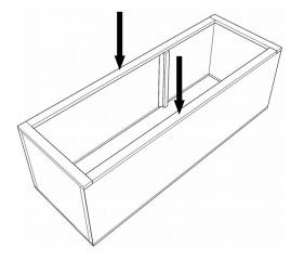
2. Attach the sides to the top and bottom using supplied screws. Be sure to align them correctly so the shelves can be installed.
