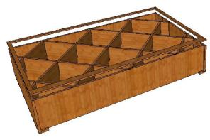
STEP 5. ATTACH (1)  $2\frac{1}{4}$ " x  $63\frac{3}{4}$ " FACE TRIM TO BOTTOM OF BIN, (1)  $1\frac{1}{4}$ " X  $63\frac{3}{4}$ " FACE TRIM TO TOP & (1ea.)  $1\frac{1}{4}$ " X  $36\frac{4}{4}$ " FACE TRIM TO EACH SIDE OF BIN w/ FINISH NAILS, STAND UPRIGHT
