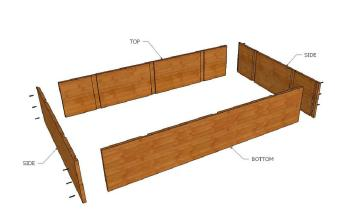
STEP 1. ATTACH TOP AND BOTTOM TO BOTH SIDES WITH (6) SCREWS AS SHOWN
