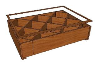
STEP 5. ATTACH (1)  $2\frac{1}{4}$ " x  $54\frac{3}{4}$ " FACE TRIM TO BOTTOM OF BIN, (1)  $1\frac{1}{4}$ " X  $54\frac{3}{4}$ " FACE TRIM TO TOP OF BIN AND (2)  $1\frac{1}{4}$ " X  $36\frac{1}{4}$ " TO SIDES w/FINISH NAILS.
