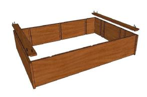
STEP 2. ATTACH (1) LEFT & (1) RIGHT CLEAT w/ SCREWS WineRacks.com Phone 888.687.2517 Fax 845.658.5309
