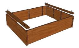
STEP 2. ATTACH (1) LEFT & (1) RIGHT CLEAT w/ SCREWS
