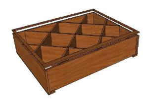
STEP 5. ATTACH (1)  $2\frac{1}{4}$ " x  $50\frac{1}{2}$ " FACE TRIM TO BOTTOM OF BIN, (1)  $1\frac{1}{4}$ " X  $50\frac{1}{2}$ " FACE TRIM TO TOP OF BIN AND (2)  $1\frac{1}{4}$ " X  $36\frac{1}{4}$ " FACE TRIMS TO SIDES w/FINISH NAILS.
