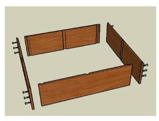
STEP 1. ATTACH (2) SIDES TO THE TOP & BOTTOM w/ SCREWS. ENSURE SLOTS ON SIDES ALIGN.
