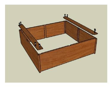
STEP 2. ATTACH (1) LEFT & (1) RIGHT CLEAT w/ **SCREWS**
