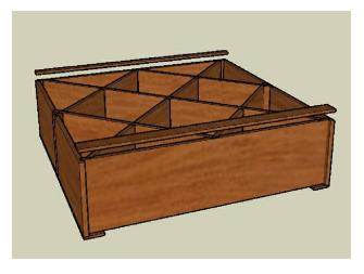
STEP 5. ATTACH (1)  $2\frac{1}{4}$ " x  $41\frac{1}{4}$ " FACE TRIM TO BOTTOM OF BIN, (1)  $1\frac{1}{4}$ " X  $41\frac{1}{4}$ " FACE TRIM TO TOP OF BIN w/ FINISH NAILS.
