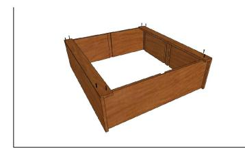
STEP 2. ATTACH (1) LEFT & (1) RIGHT CLEAT w/ SCREWS
