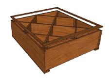
STEP 5. ATTACH (1)  $2\frac{1}{4}$ " x  $36\frac{3}{4}$ " FACE TRIM TO BOTTOM OF BIN, (1)  $1\frac{1}{4}$ " X  $36\frac{3}{4}$ " FACE TRIM TO TOP & (1ea.)  $1\frac{1}{4}$ " X  $36\frac{1}{4}$ " FACE TRIM TO EACH SIDE OF BIN w/ FINISH NAILS. STAND UPRIGHT
