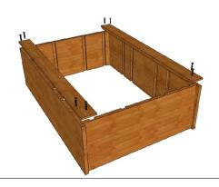
STEP 2. ATTACH (1) LEFT & (1) RIGHT CLEAT w/ SCREWS
