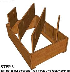
FLIP BIN OVER. SLIDE (2) SHORT SHELVES & (2) LONG SLELF INTO SLOTS AS SHOWN. ENSURE SHELF NOTCHES FACE UP AND ALIGN.
