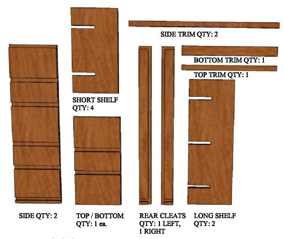
ITEMS SUPPLIED BUT NOT SHOWN: 24 - WOOD SCREWS 1 TUBE OF GLUE NAILS FOR FACE TRIM WineRacks.com Phone 888.687.2517 Fax 845.658.5309
