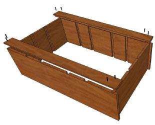
STEP 2. ATTACH LEFT AND RIGHT CLEATS TO BACK OF BIN WITH GLUE AND SCREWS AS SHOWN
